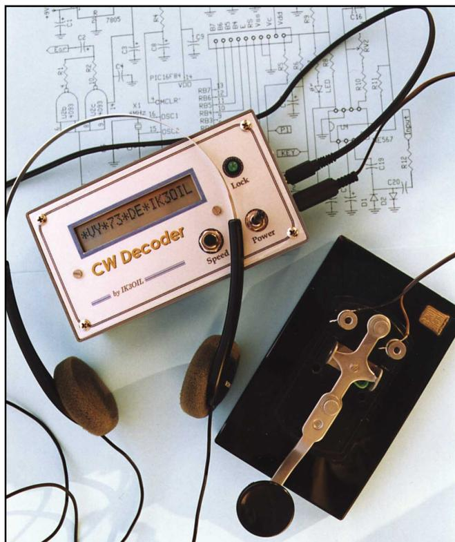
The asterisks appearing at the interword spaces are generated by sending a bogus Morse character. This display was generated using the straight key and as shown here, interword spacing is turned off.
