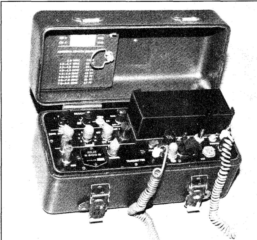
*The Delco 5300B, the CIA version of the PRC-64 transceiver.*
