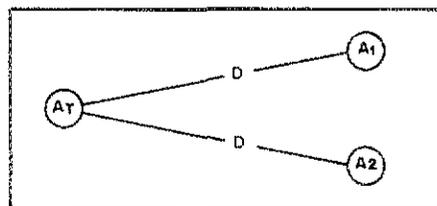
Fig. 2 — If both receiving antennas are an equal distance (D) from the transmitting antenna, there will be no difference in the phase angles of the signals in the receiving antennas; therefore, the detector will not detect any phase modulation, and the audio tone will disappear from the output of the detector.
