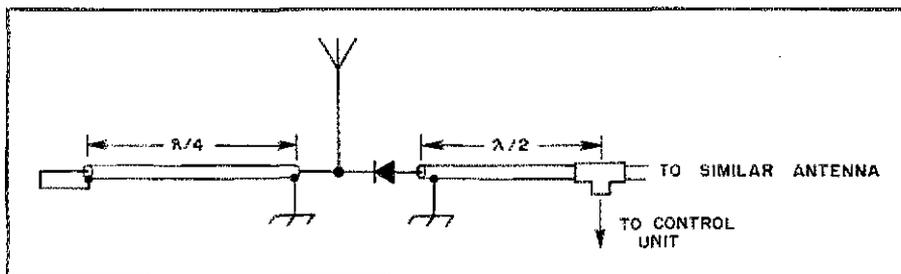
Fig. 7 — Another variation of the basic design. Here, a shorted quarter-wavelength section of coaxial cable replaces the rf choke at the antenna.
