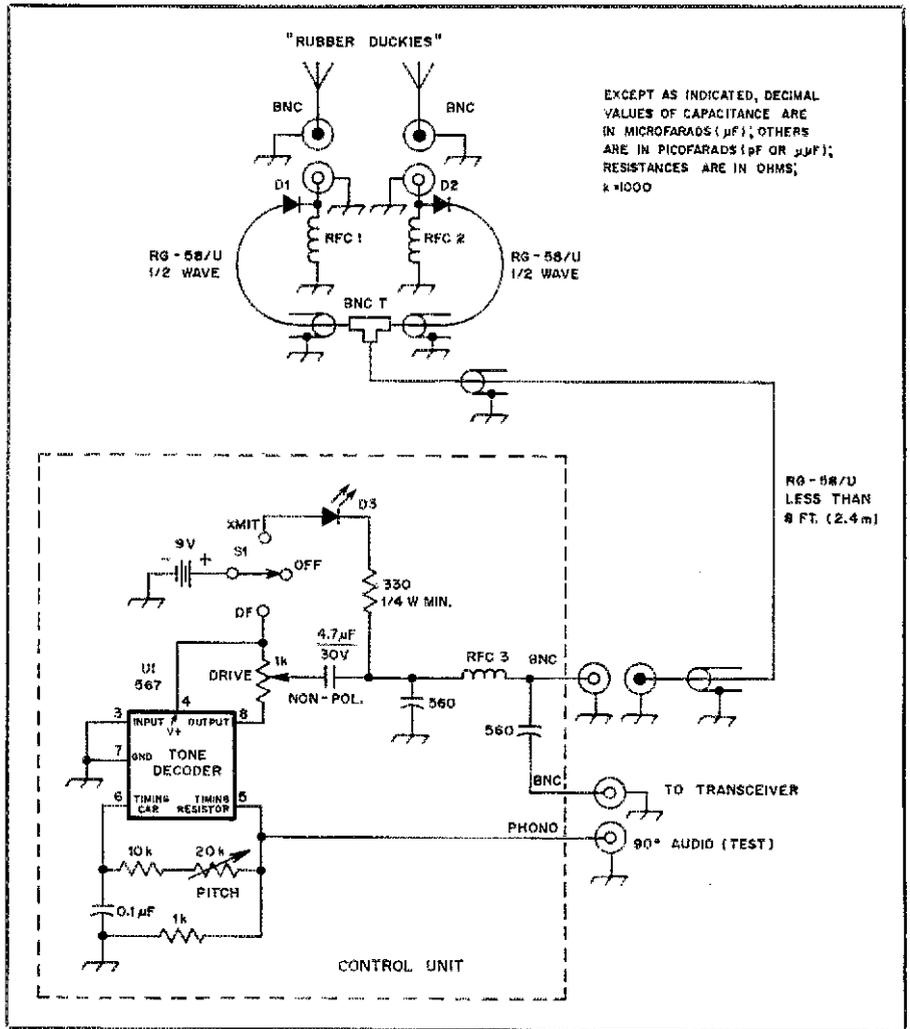
Fig. 4 — Schematic diagram of the DDDF circuit. Construction and layout are not critical. Components inside broken lines should be housed inside a shielded enclosure. Most of the components are available from Radio Shack, except D1, D2, the antennas and RFC1-RFC3, which are discussed in the text. S1 — See text.
