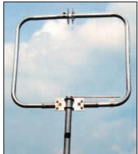
Figure 2—After: The 6 meter squalo, ready for action.
